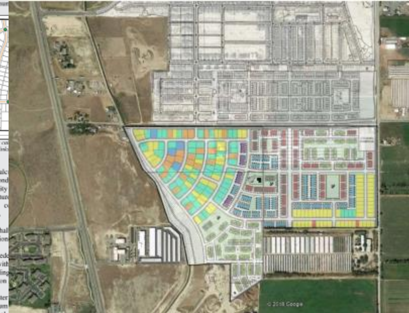
Figure 27. Example connectivity index calculation. This example shows 23 links divided by 13 nodes, resulting in a connectivity index of 1.77.
