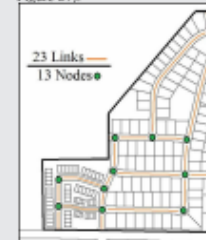
Figure 27. Example connectivity index calculation. This example shows 23 links divided by 13 nodes, resulting in a connectivity index of 1.77.
